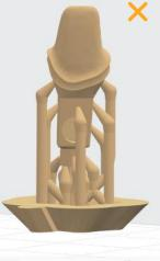
Printing on supports is also possible, and is recommended in cases where dies have small pin diameters (less than 3 mm).
